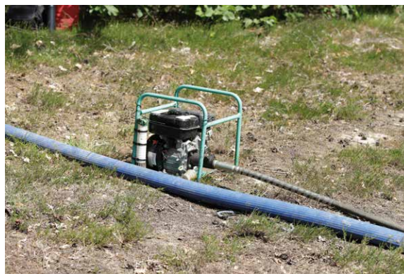
Figure 82. Pompe thermique. Photo ©CDPNE
